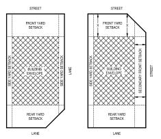
Figure 4.1: Corner Cut-off Lot Minimum Yard Dimensions
