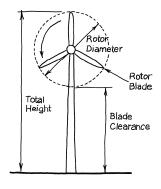
**Blade** means an element of a wind energy system rotor, which acts as a single airfoil, thereby extracting kinetic energy directly from the wind.
