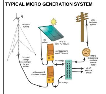
Figure 1. Typical wiring connections for a grid-connected micro wind and solar PV system. (Source: Modified from an unknown source. Gratefully included in this document.)
